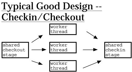
There are many worker objects. Each "checks out" data from a shared input stage, but is then able to proceed independently for the most part -- not accessing (locking) shared memory. When it's finished, the worker typically needs to "check in" its results to some sort of shared output stage. Parallelism will work best if the checkin/checkout operation is small compared to the work each worker can do.
